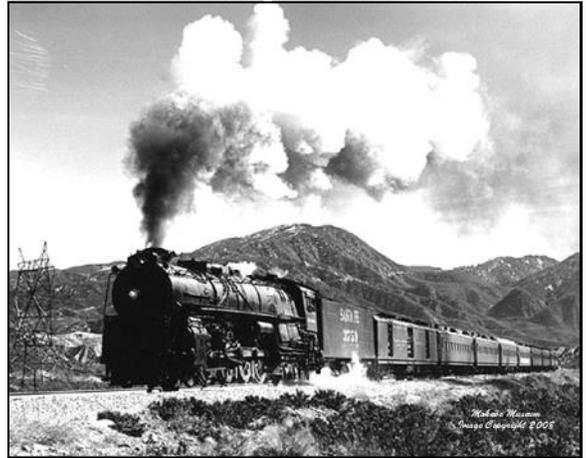
3759 was delivered in 1928 as a 3751 class 4-8-4 passenger locomotive. Originally a coal burning locomotive with 73-inch drivers, the fleet was converted to oil in 1936 and rebuilt between 1938 and 1941 with 80-inch drivers. Its regular passenger run was from Los Angeles to Kansas City, with Kingman as a water stop on the way back to Los Angeles. Retired in 1953, the engine had traveled over 2,585,000 miles.
